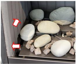
Ensure that the ceramic panels are pushed hard to the side and rear
