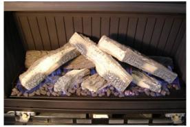
Place the granules evenly around and in the gaps between the logs. DO NOT place the granules near the flame rods or the pilot (circled area above) as this will cause blockages in the appliance.
