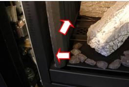
Ensure that the Ceramic Panels are pushed hard to the Side and Rear
