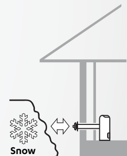
Keep snow away from the flue terminal
