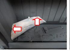
Ensure left hand log is pushed hard against LH side and Rear Ceramic Panels
