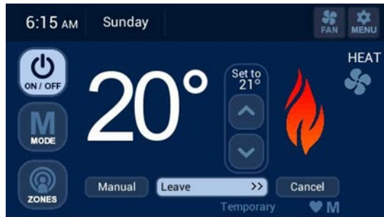
Diagram 6: Heating Temperature Override
