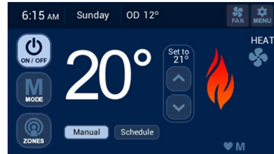
Diagram 38: Outdoor Temperature Display
