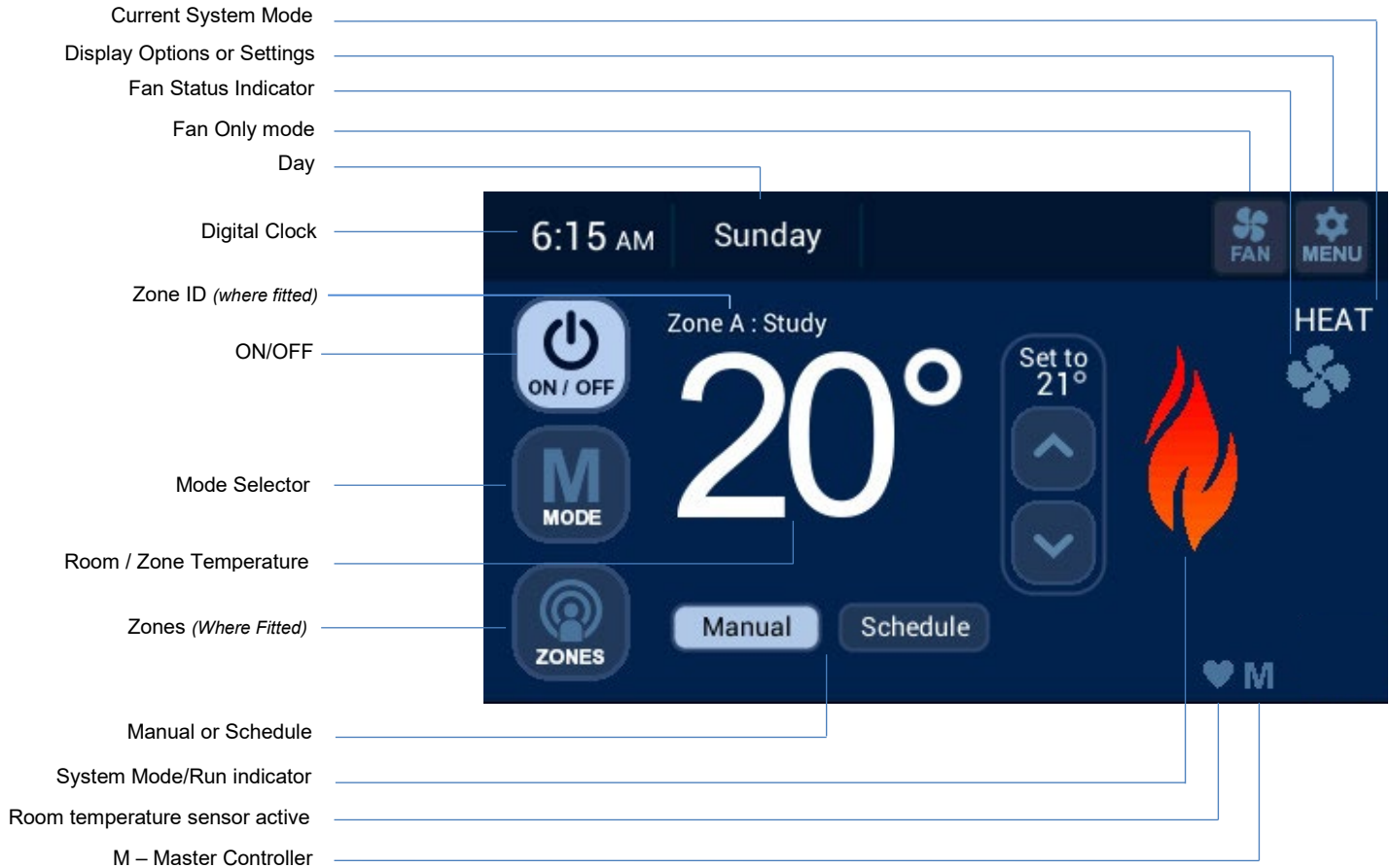
Diagram 1: Heating screen in Manual Operation
