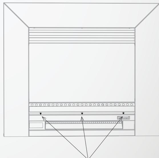
Traditional Frame secured to unit with three screws
