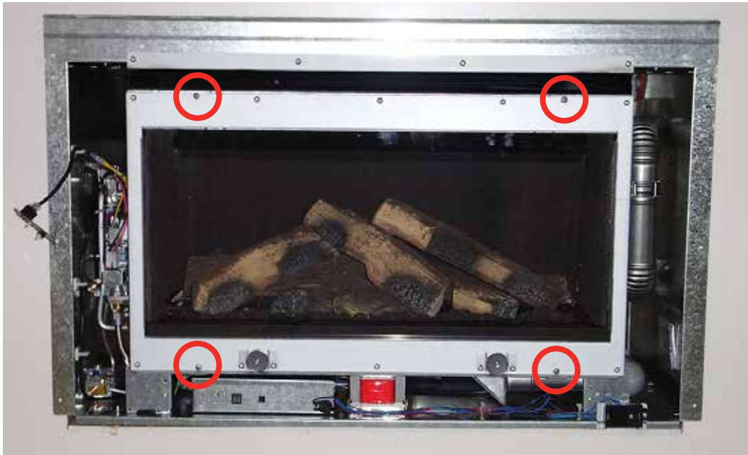
Front panel of the Evolve showing the four screw positions for removing and replacing the glass panel
