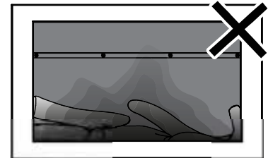
Soot build up
