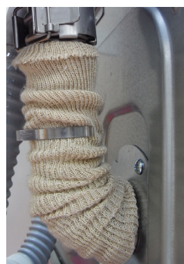
Securing the protective sock
