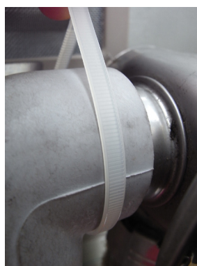
Combustion air hose attachment
