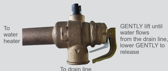
How to operate the easing gear
