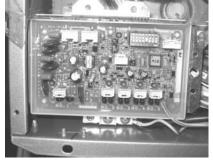
2) Connect the connector from Communication Cable to socket No. 1 on Control Board.
