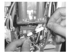
7) After making all of the connections to the Control Board, tighten all of the cable ties used to secure the Communication Cables. Ground all the Communication Cables.
