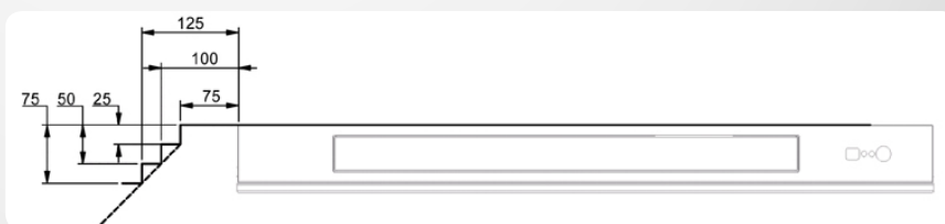
Arriva surround clearances
