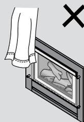
Do not allow curtains or other combustible materials to come into contact with the appliance.
