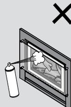
Do not spray aerosols while the appliance is operating. Most contain butane gas which can be a fire hazard if used near the appliance.
