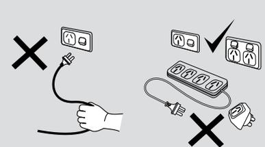
Do not unplug the appliance while it is operating. Do not use power boards or double adaptors to operate this appliance.
