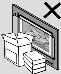
Do not restrict warm air discharge by placing articles in front of the appliance.
