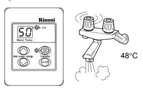
There is no need to turn the Temperature Controller(s) off after use. However, if you prefer to turn the Temperature Controller(s) off, selected temperatures will be stored in the system memory at all times whilst mains power remains connected.
