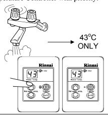
Depending on the weather conditions and the length of the pipe between the hot water unit and the tap in use, there may be a variation between the temperatures displayed at the Temperature Controller(s) and the temperature of the water at the tap.
