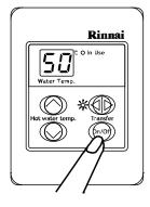
If a temperature is higher than 50°C, and has been selected at the Kitchen Controller and then priority of temperature selection is transferred to a Bathroom Controller and back again, the temperature on the Kitchen Controller will drop to 50°C. This is a safety feature.
