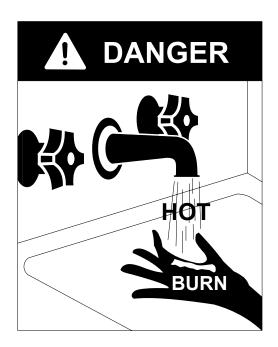
Water temperatures over 50°C can cause severe burns instantly or death from scalds.
