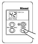
The yellow ON indicator will glow on the Temperature Controller. This indicates that the hot water unit is ready to supply hot water when a tap is open.
