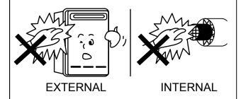
On cold days steam may be discharged from the flue outlet. This is normal with a high efficiency appliance and does not indicate a fault.
