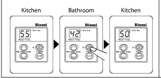
Do not push the ON/OFF button on the Kitchen Controller after having transferred priority of temperature selection to the Bathroom Controller as the system will no longer heat the water.
