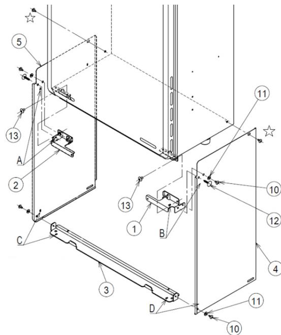
4. Attach the front lower bracket to the right and left side panels with the truss and tapping screws (10), and plastic washers (11). There is one screw and washer for each side. Align marks 'C' (left hand side) and 'D' (right hand side).
