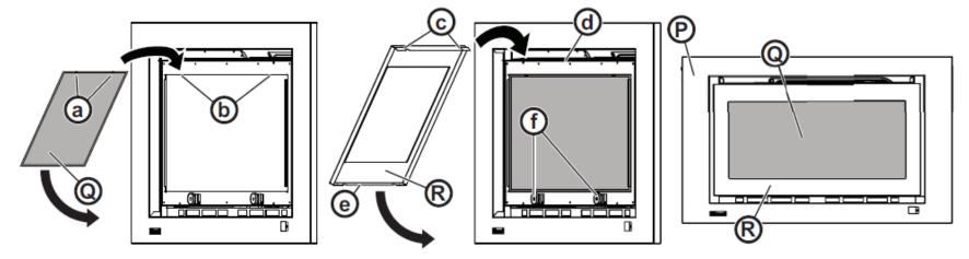
3. Rotate the bottom of the inner fascia (a) in towards the engine body allowing the magnets (b) to secure both the inner fascia and the dress guard to the heater engine.
