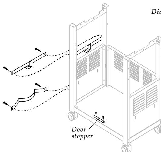
7. Attach the door bracket to the lower holes in the front legs with the end tabs pointing upward and the flange to the rear, pointing downward. Use two (2) of the  $\frac{1}{4}$ " x  $\frac{1}{2}$ " Phillips-head screws. Do not fully tighten. Refer to diagram 4.
