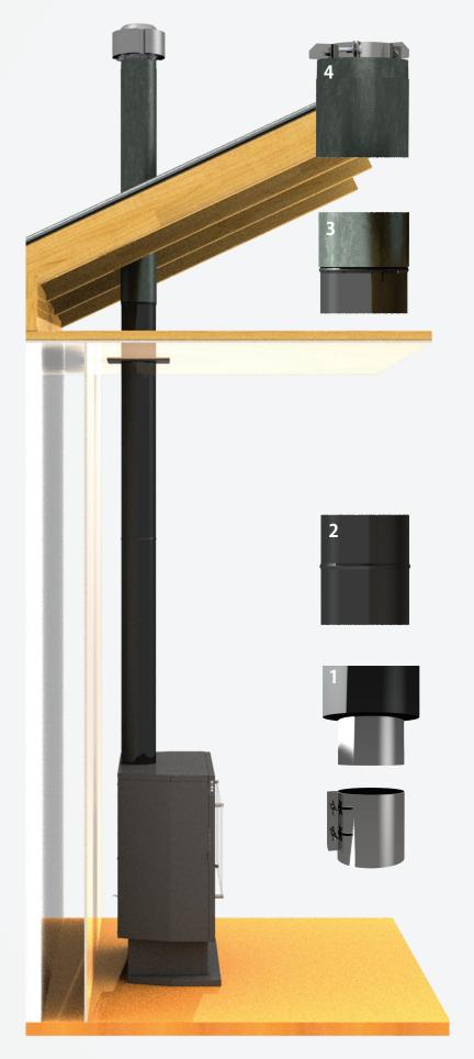
**1.** Install the clamp sleeve into the flue spigot of the fire—acts as a spacer to disengage the flue when needed.
