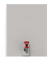
The Rinnai Boil & Brew is a permanently plumbed, wall-mounted electric water heater with an insulated hot water container. Water is heated by an electric heating element and the temperature is controlled by a thermostat. As boiling water is drawn off, the unit refills with cold water. Any steam generated during the heating cycle is condensed and retained within the unit.
