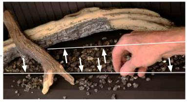
with arrows below). This gap is required for secondary air to get to the burner.
