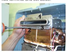
4. Install the diverter onto the flue terminal, reinsert screws and tighten.
